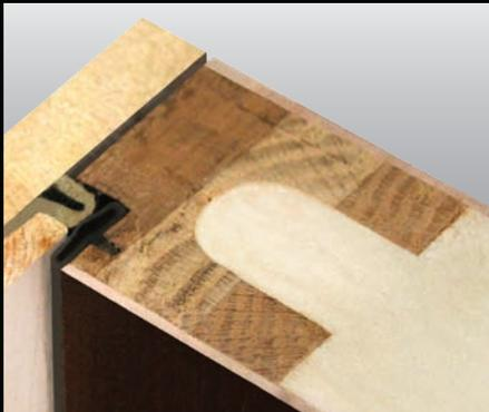
We engineered a channel in the side rails and header of the door to **allow for a larger energy efficient polyurethane core**. Our computer-controlled process fills every crevice with the foam barrier material resulting in a level of energy efficiency unparalleled in the industry.
