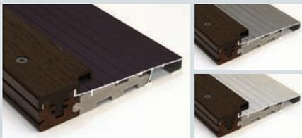
Our exclusive Bronze **Sahara™ heavy-duty extruded threshold** has a 2¾" wide thermal barrier wood-look riser that will not warp or rot while providing excellent energy efficiency. On entry systems with sidelites, our continuous threshold improves structural integrity and helps prevent rotting. Also available in Anodized Nickel or Mill finish.
